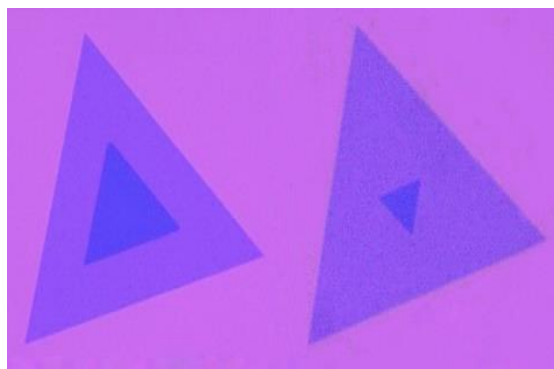
Figure 1: Optical image of CVD-grown WSe 2 bilayer flakes
